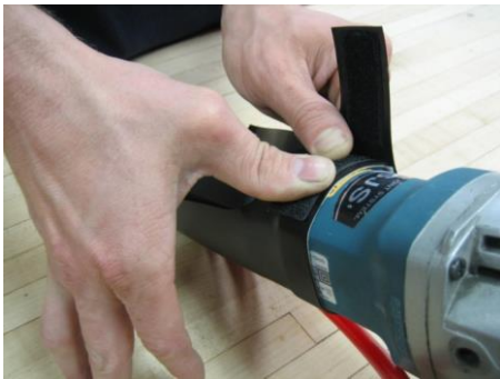
FIGURE 6 – Spray Skirt Installation
