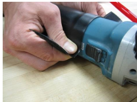
FIGURE 5 – Spray Skirt Installation
