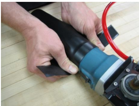
FIGURE 4 – Spray Skirt Installation
