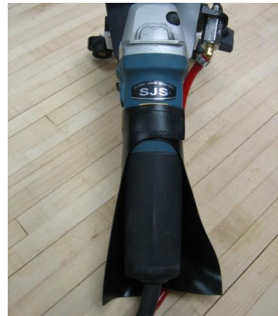
FIGURE 7 – Spray Skirt Installation Complete
